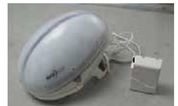
9. Remove the tape covering the air inlet channel of the Filter Cover Cap.
