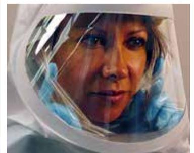
12. Pull back of shroud up, over, and down behind helmet. Slide fingers between face and cuff on both sides from chin to temples to ensure a slight Cuff-to-Face tension.\*
