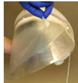
3. Remove a DLC from the DLC dispensing box and attach the DLC Lens, with the DLC cuff facing the inside to the helmet. Remove the DLC Protective film.
