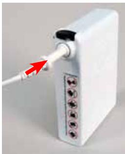
4. Connect the Helmet Power Cord to the Battery. Push the Power Cord Connector into the Battery Receptacle until the Secure Connection audibly clicks.
