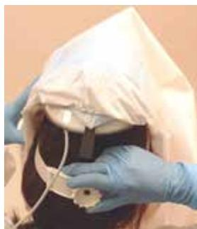
13. Secure Helmet by tightening Ratchet Knob as tight as comfortably possible, while ensuring stability.
