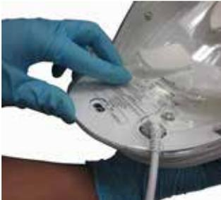
4. Push the rear edge of the Liner inward with your thumb inward. Align the rear Liner holes over the Helmet rear snaps.
