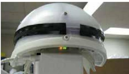
7. Lay the tape flap back down to reduce the gap back to a one inch opening. Allow the Helmet to stabilize for about a minute. Notice the Yellow LED turns on.
