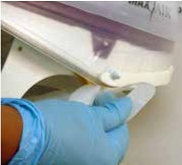
2. Attach one side of the DLC alignment hole to the Helmet side attachment post (Cuff facing inward).
