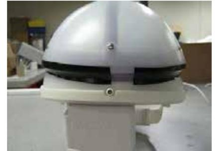
1. Start taping approximately one inch away from the front-center of the Helmet. (One inch to the side of the front Alignment post.
