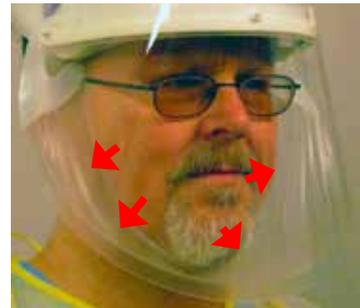
**Condition 2:** Ensure slight tension on the cuff is felt continuously while sliding the index or first finger between the cuff and the face all along the chin and up to the temples, from the right side of the face to the left.
