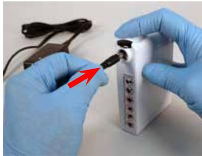
5. With the Charger connected to the mains wall power, connect the Charger Cord to the Battery. Push the Charger Cord Connector into the Battery Receptacle until it is fully seated.
