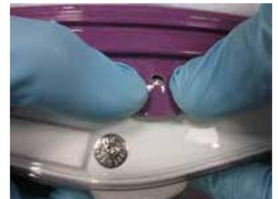
6. Snap and secure each Filter Cartridge side snap tab on to each respective Helmet side upper snap.
