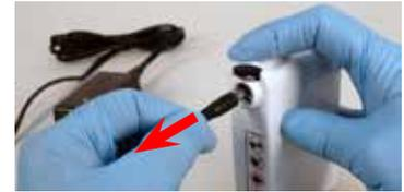
1. Connect the Charger (single and/or 6-Gang) to an appropriate grounded wall mains power source (120-240 VAC, 50-60 Hz) before connecting to the Battery(ies). The Charger green status LED should turn on.
