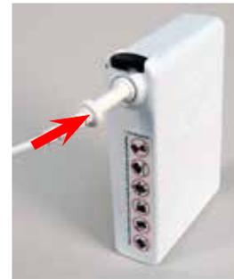
5. Connect the Helmet Power Cord to the Battery. Push the Power Cord Connector into the Battery Receptacle until the Secure Connection audibly clicks.
