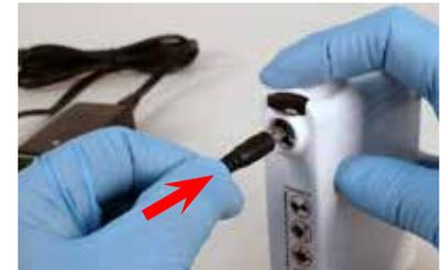
6. With the Charger connected to the mains wall power, connect the Charger Cord to the Battery. Push the Charger Cord Connector into the Battery Receptacle until it is fully seated.
