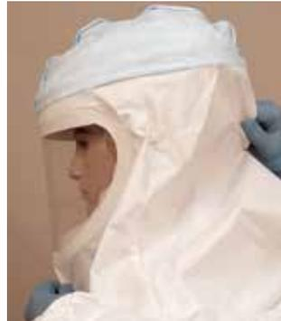
14. Ensure all Filter (blue) wrinkles above front of Lens are removed by holding shroud in front below lens and in back below filter and pulling down firmly.
