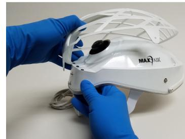
4. Lift the 2051-07 SnapOn Cage up and off the Helmet.
