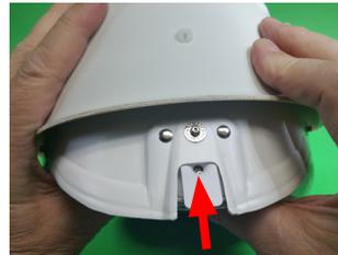
8. Pull the Hard Hat down over the back of the Helmet until its T-Tab hole is over the top rear Snap on the Helmet back.
