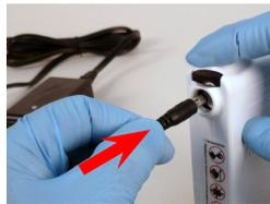
9. With Charger connected to safe power source, connect Charger Cord to the Battery. Push Charger Cord Connector into Battery Receptacle until fully seated.
