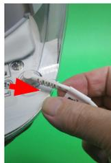
3. Align the Helmet Power Cord with the Liner Cord cutout and press the Liner rear against the Helmet.
