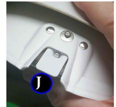
2. Assemble Hard Hat to Helmet: Locate Helmet front Mounting Adapter (E), locate Hard Hat front Mounting Hole (F); Place Adapter into Mounting Hole (G); pull Hard Hat over and down on Helmet (H) until Hard Hat T-Tab (I) is over and snaps to lower rear Helmet Snap (J).
