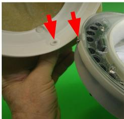
6. Locate the inside hole in the Hard Hat front Turn Clip, and the Helmet front Snap.
