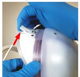
1. With one hand, hold the Helmet and FCC with the thumb against the FCC and the fingers on the inside of the Helmet. With the other hand, pull up on the FCC T-Tab and unlatch it from the Helmet FCC Rear Bottom Snap.
