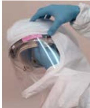
4. Pull Hood down until the front Hood Snap is over the center Helmet Snap.
