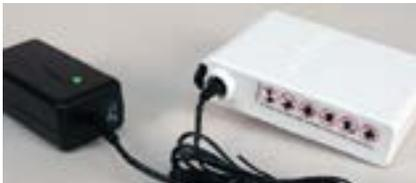
1. Obtain a fully charged battery. (Charger LED should be green after battery is connected to charger for more than 10 seconds.)
