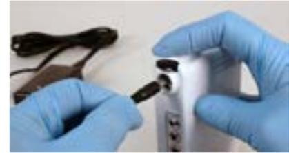
12. Connect a powered on Battery Charger connector to the Battery. Push connector into Battery receptacle fully - Do NOT push down on the Battery Secure Lock (Black) button.
