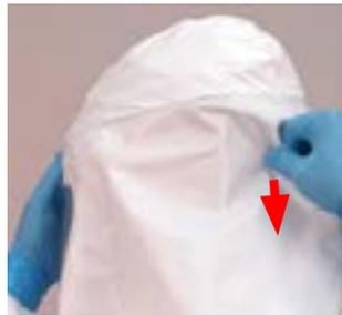
11. Continuing process of 14, pull Hood all the way down so that Hood Filter (top) is fully down on Helmet.
