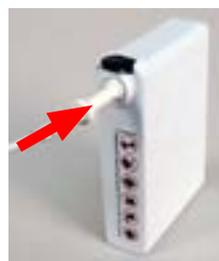
4. To begin air flow, insert Helmet Power Cord Connector into Battery Connector receptacle until the Secure Connection audibly clicks.
