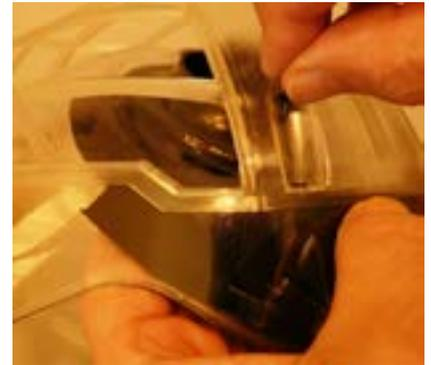
2. Using a thin, flat blade (small screwdriver etc.) pry each rivet up and out of the Cage.
