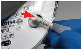
1. Ensure the Power Cord is aligned with the Liner Cord cutout.
