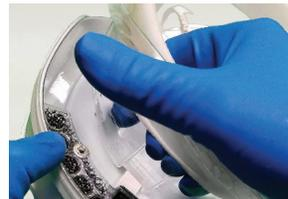
3. With thumb against bottom front of Helmet, pull fingers down and push thumb up to disengage Front Snaps.
