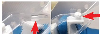
2. Insert Side Tab Rear Button into Rear Side Tab slot from underneath, then push all the way backward.
