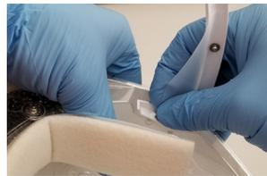
3. Place ChinBar Front Button into front Liner Button Slot.
