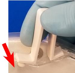
1. Push Front Button inward to remove from Front Slot.
