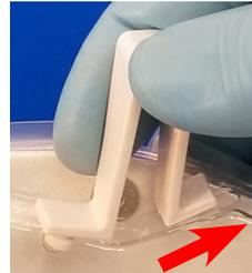
2. Push Rear Button rearward to large hole end of Rear Slot; then pull Side Tab up to remove from Rear Slot, and remove Tab from Liner. Repeat for other side.
