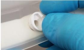
1. From inside the FCC, place a new Front Lens Mount into the front hole on the FCC.
