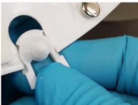
1. Grasp a Side Lens Mount between thumb and forefinger and slide it into the Side Lens Mount slot in the FCC.
