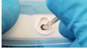
2. Push the Front Vent Clip fully out of the Front Lens Mount.
