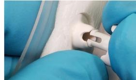
3. From outside the FCC, position the legs of a Front Vent Clip into the front opening of the Front Lens Mount.
