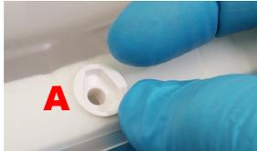
2. Position the Front Lens Mount as shown at A.
