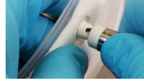
4. Bracing the front of the FCC from the inside, push the screddriver inward with controlled force to push the Front Lens Mount out of the FCC.
