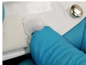
2. Press the Side Lens Mount fully up into the slot as shown in A.
