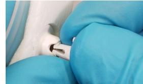
4. Compress the legs of the Front Vent Clip by wedging them into the opening of the Front Lens Mount.
