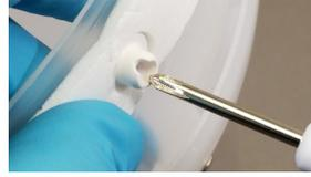
3. From outside the FCC, insert the Phillip blade through the Front Lens Mount.
