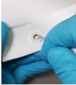
2. From inside the HH, pinch the legs of the Side Turn Clip together with the MAXAIR Screwdriver flat blade, and push the turn Clip out of the HH Skirt.
