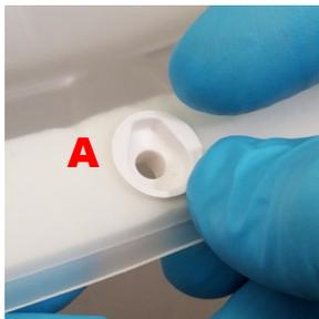
2. Position the Front Lens Mount as shown at A.
