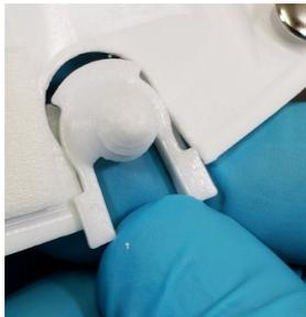
1. Grasp a Side Lens Mount between thumb and forefinger and slide it into the Lens Mount slot in the HH.
