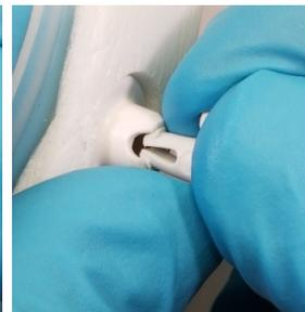
4. Compress the legs of the Front Vent Clip by wedging them into the opening of the Front Lens Mount.
