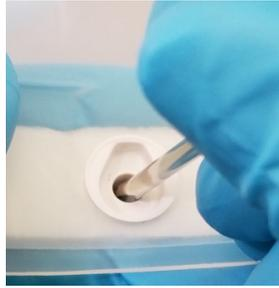
2. Push the Front Vent Clip fully out of the Front Lens Mount.
