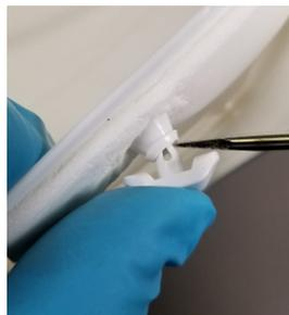
3. From outside the HH, use the screwdriver flat plat to aid in positioning the legs of a Side Turn Clip into the front opening of the Side turn Clip Base.
