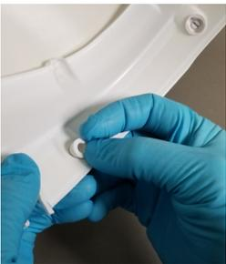
1. From inside the HH, place a new Side Turn Clip Base into the round side hole on the HH.
