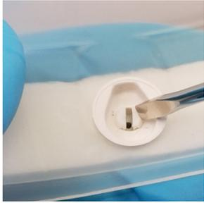
1. From inside the HH, pinch the legs of the Front Vent Clip together with the MAXAIR Screwdriver flat blade.
