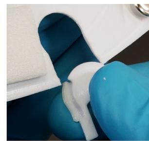
2. Grasp the Side Lens Mount between thumb and forefinger and pull down and away from the HH.
