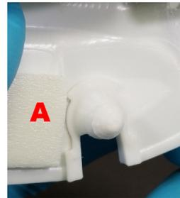
2. Press the Side Lens Mount fully up into the slot as shown in A. Alternatively, use the Screwdriver Flat Blade as leverage to push the Lens Mount fully into the Lens Mount Slot.
