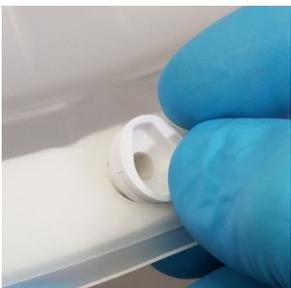
1. From inside the HH, place a new Front Lens Mount into the front hole on the HH.
