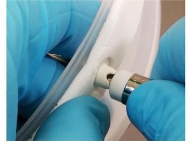
4. Bracing the front of the HH from the inside, push the screddriver inward with controlled force to push the Front Lens Mount out of the HH.
