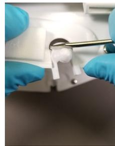
Alternative to step 2, position both thumbs at bottom edge of HH Skirt for support, and use the screwdriver flat blade on top of the protruding post and press down to remove the Lens Mount.
