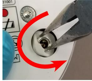
3. Using a standard pair of Needle-nose pliers, grasp opposite flat sides of the Hex Nut and loosen by turning counterclockwise.
