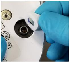
1. Place a new TurnLock connector over the Power Jack.
