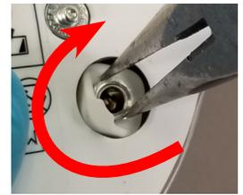
4. Use the Needle-nose pliers to tighten the Hex Nut firmly onto the Power Jack.
