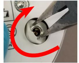
4. Use the Needle-nose pliers to tighten the Hex Nut firmly onto the Power Jack.
