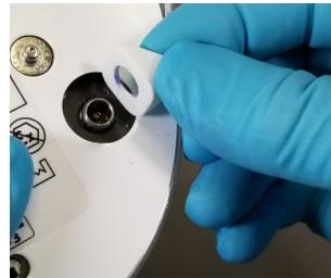
6. Lift the old TurnLock connector off its mounting on the Power Jack and discard appropriately as potentially contaminated waste.
