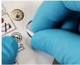
2. Fully seat the Turn-Lock connector down on to the Power Jack.
