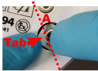
3. Start threading a Hex Nut over the TurnLock connector and on to the Power Jack by turning it clockwise.
