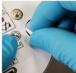
5. Grasp the old TurnLock connector with fingers. If old connector is broken it may be necessary to grasp it with the Needle-nose pliers.
