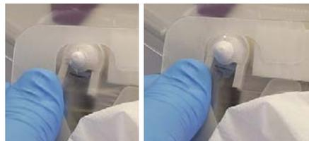
5. That side DLC Mounting Hole centered over the FCC side Mounting Post, press the DLC down fully onto the Mounting Post. An audible click indicates the DLC is properly around and down securely on the Mounting Post.
