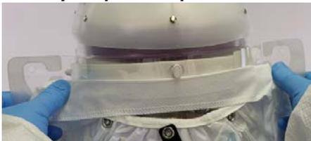
4. With thumbs pressing the DLC against the FCC front white foam strip, press and slide your thumbs down each DLC side until you can grasp each end of the DLC at the Flappers.
