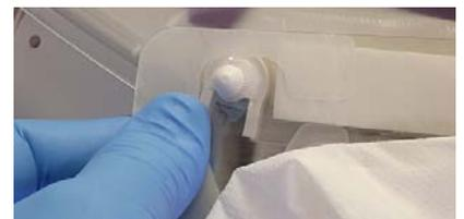
6. Press the DLC tightly against the FCC to secure the Mounting Hole onto each Mounting post. (You will hear an audible "click" when properly secured).
