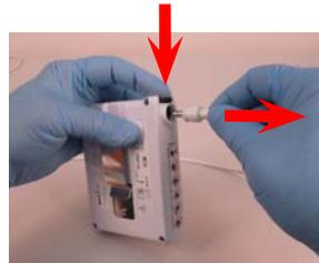
7. Disconnect the Helmet Power Cord from the Battery - push the Secure Connection Button down, pull Cord Connector out, release the Button.
