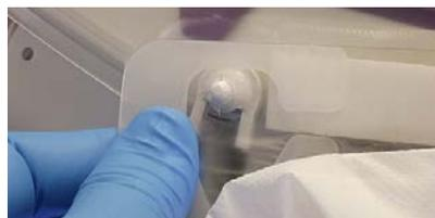
5. Pull each DLC side down towards the Helmet back and tightly against the white foam strip, position each side DLC Mounting Hole as centered as possible over each respective FCC side Mounting Post.
