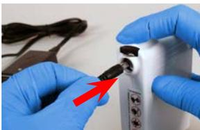
9. With Charger connected to safe power source, connect Charger Cord to the Battery. Push Charger Cord Connector into Battery Receptacle until fully seated.
