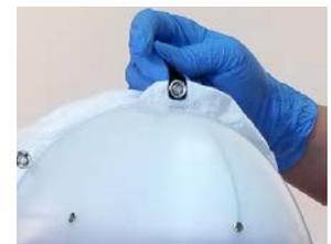
9. Pull Shroud over and down the back of the Helmet.
