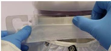
4. The DLC Front Alignment Hole secured, grasp one DLC end by the Flapper and stretch it tautly until that side Mounting Hole is over that side Mounting Post.
