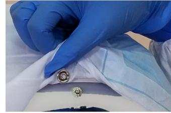
11. Snap and secure left Rear Side Snaps between Shroud and FCC. Then repeat on right Rear Side Snaps.
