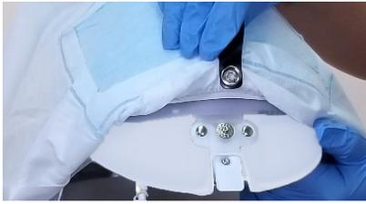
10. Use Pull Tap to position Shroud Rear Snap over FCC Rear Snap; snap and secure.
