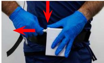
7. Disconnect the Helmet Power Cord from the Battery - Press down on the Secure Lock (Black) Button to release, then pull the cord connector out from the Battery connection receptacle.
