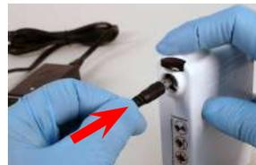
12. With Charger connected to safe power source, connect Charger Cord to the Battery. Push Charger Cord Connector into Battery Receptacle until fully seated.
