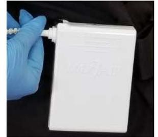
8. Connect Helmet Power Cord to Battery. Push Power Cord Connector into Battery Receptacle until Secure Connection audibly clicks.
