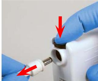
11. Press down on the Secure Lock (Black) Button to release, then pull the cord connector out from the Battery connection receptacle.
