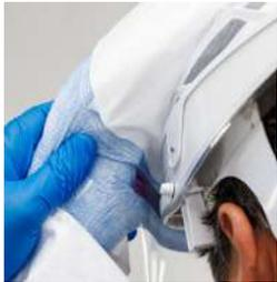
5. Unsnap each side attachment and continue moving rolled Hood forward and off front Helmet Mounting Post.
