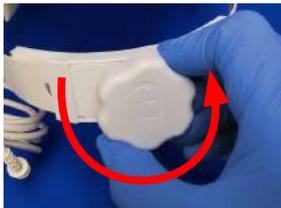
9. Loosen the ratchet adjustment knob counter-clockwise to ensure the Helmet will easily fit over the head.
