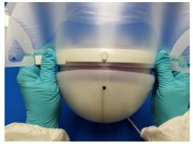
4. With thumbs pressing the DLC against the FCC front white foam strip, press and slide your thumbs down each DLC side until you can grasp each end of the DLC at the Flappers.
