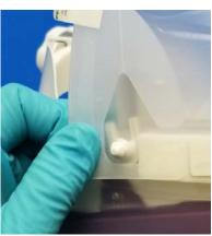
6. Press the DLC tightly against the FCC to secure the Mounting Hole onto each Mounting post. (You will hear an audible "click" when properly secured).
