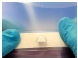
2. Align the FCC front TurnClip horizontally, snap the DLC Front Alignment Hole over the TurnClip, then position the TurnClip vertically to lock the DLC in place.
