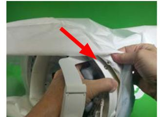
5. Use the black pull tab to pull the Shroud up over the Hard Hat front and back towards the rear.
