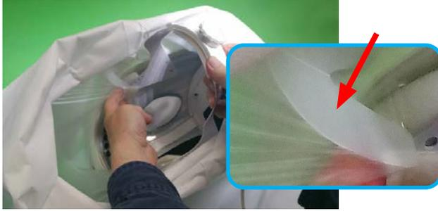
2. Ensure the Cuff Flappers are out away from the Lens and over the foam pads on the Liner sides.
