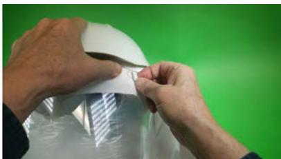
1. Securely attach one set of side Lens holes (2) over one side Hard Hat Turn Clip and Mounting Post. Secure Turn Clip vertically.
