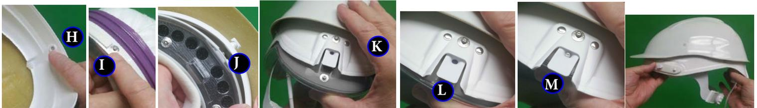
3. Re-Assemble Hard Hat to Helmet: Locate Hard Hat front Mounting Hole (H), locate Helmet front Mounting Snap (I); Place Mounting Snap into Mounting Hole (J); pull Hard Hat over and down on Helmet (K) until Hard Hat T-Tab (L) is over and snaps to lower rear Helmet Snap (M).
