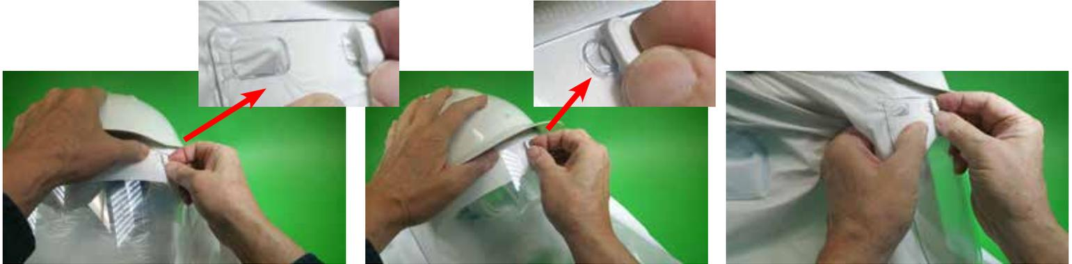
1. Securely attach one set of side Lens holes (2) over one side Hard Hat Turn Clip and Mounting Post. Secure Turn Clip vertically.
