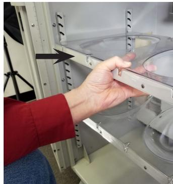
2. With the Shelf at the desired height, move the Shelf backward to engage the Pins into the Slots.
