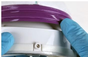
2. Using the bottom step on the Filter Cartridge front plastic Retainer Ring, pull the Filter Cartridge up off the Helmet front.
