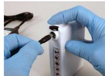
3. Connect a powered on Battery Charger connector to the Battery. Push connector into Battery receptacle fully - Do NOT push down on the Battery Secure Lock (Black) button.
