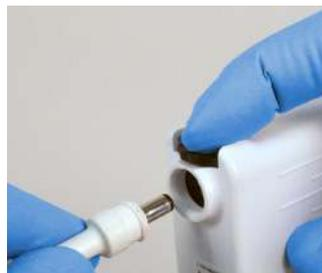
2. Disconnect the Helmet Power Cord from the Battery - Press down on the Secure Lock (Black) Button to release, then pull the cord connector out from the Battery connection receptacle.
