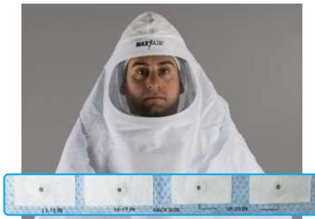
9. Note the four snap positions on the Necktie. Choose the position that provides the wearer a comfortable fit, ensures the hood is within about an inch of the neck for a good fit, and allows freedom of head movement.
