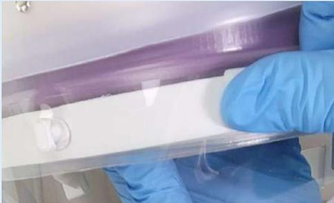
While pressing Lens against FCC Foam Strip, slide fingers along the Lens to one side and snap the DLC side Lens hole over the FCC side Lens mount. Repeat for other side.
