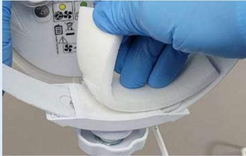
The Rear Comfort Strip is closed cell foam and may be cleaned with a decon wipe and reused. To remove, peel up one end from the Liner rear Headband and pull it away and off the Headband.
