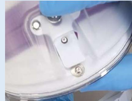
Ensure the T-Tab is fully secure on the Helmet Snap – should feel/hear a slick click when secured.
