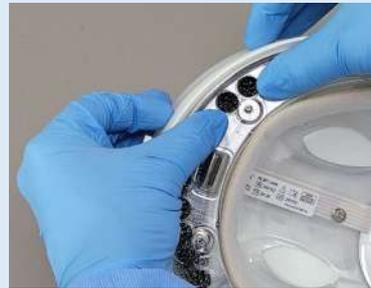
Secure both top Liner snap holes to top Helmet snaps
