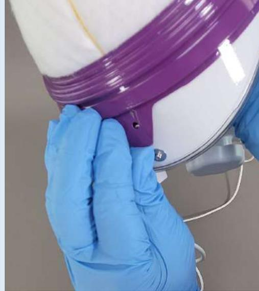
Lift rear snap tab off of Helmet snap and continue lifting Filter Cartridge up and off Helmet.
