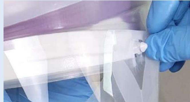
While pressing Lens against FCC Foam Strip, slide fingers along the Lens to one side and snap the DLC side Lens hole over the FCC side Lens mount. Repeat for other side.
