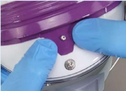
Secure Cartridge rear by pressing rear tab down on snap
