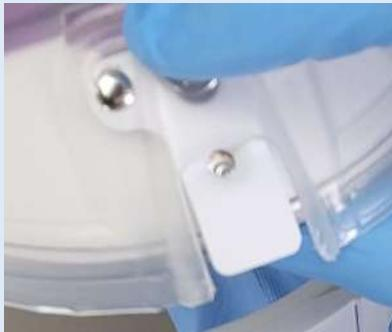
Pull the FCC fully down on the Helmet to align the FCC T-Tab snap hole over the Helmet rear bottom Snap
