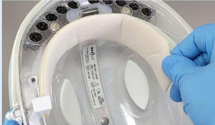
Remove the Front Comfort Strip by peeling up one end of the Strip and continue pulling to remove completely from the Headband.
