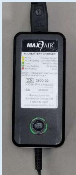
Connect the battery to the to a powered on 2600-02<sup>1</sup> Charger to re-charge. Insert the Charger Connector all the way into the Battery Connector. Push in firmly until you feel the Charger Connector “hit bottom” of the Battery Connector.
