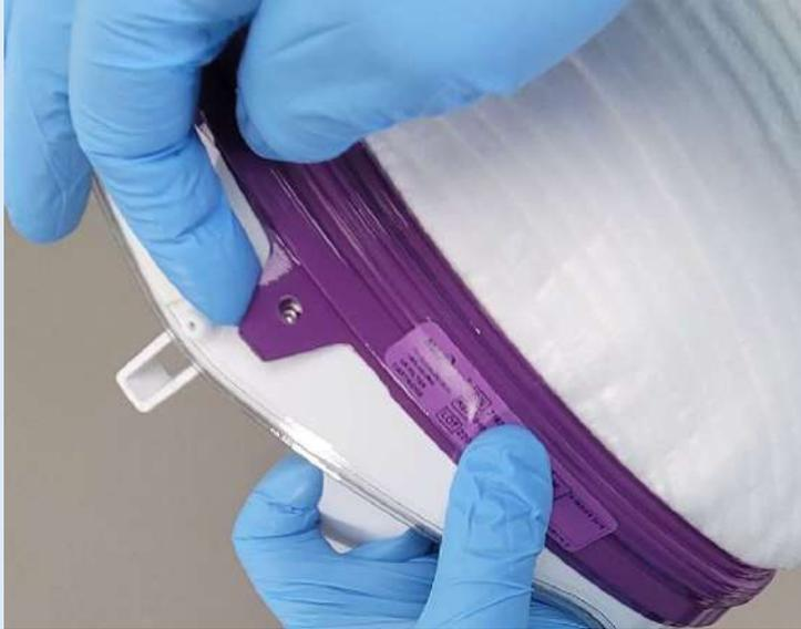
Gently lift each Cartridge side snap tab off of Helmet snap.
