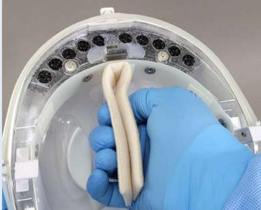
Attach the center of a new Comfort Strip to the center Headband Velcro.
