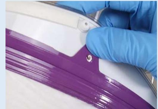
Secure both left and right side tabs by pressing tabs down on snaps
