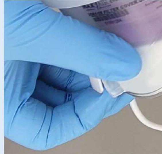
With the other hand, lift up on FCC T-Tab to unlatch it from Helmet Snap.
