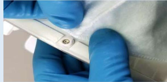
Place Filter Cap over Helmet and align its center front bottom just above Helmet Front Lens Mount and press adhesive firmly to Helmet.
