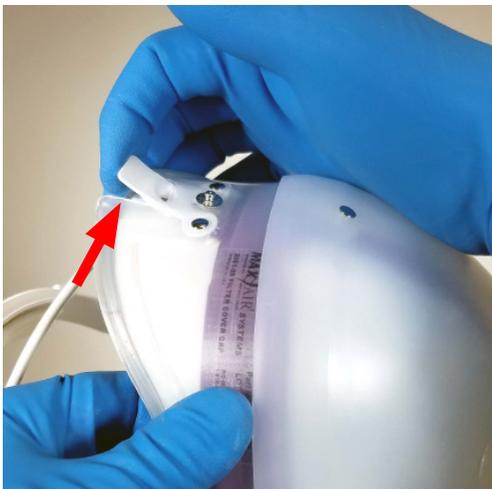
1. With one hand, hold the Helmet and FCC with the thumb against the FCC and the fingers on the inside of the Helmet. With the other hand, pull up on the FCC T-Tab and unlatch it from the Helmet FCC Rear Bottom Snap.
