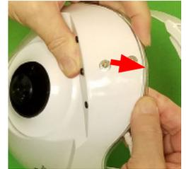
5. Ensure the Liner outer edges curls up and over the Helmet edge, all around the Helmet.
