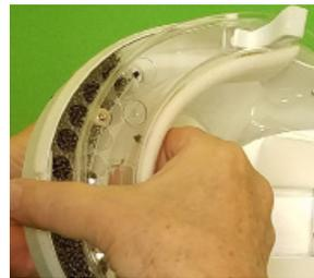
3. With thumb against bottom front of Helmer, pull fingers down and push thumb up to disengage Front Snaps.
