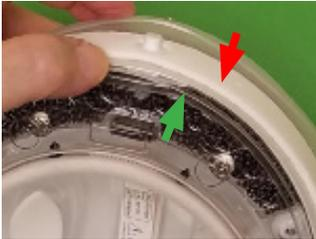
1. Place Liner front (green arrow) under Helmet front (red arrow) to align Helmet Snaps with Liner Snap Holes.
