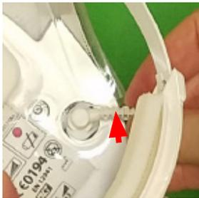
1. Ensure the Power Cord is aligned with the Liner Cord cutout.
