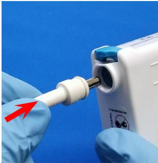
1. Connect the Power Cord connector to the Battery. Do NOT push down on the Battery Secure Lock (Black) button.
