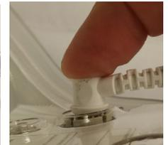
3. Place the newer Power Cord-to-Helmet Connector into the Helmet receptacle and push in until it is firmly seated.
