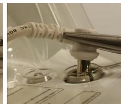
2. Firmly lift the Power Cord-to-Helmet Connector up and out of the Helmet receptacle.
