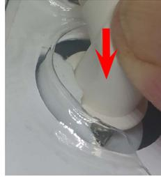
2. Push Cord connector fully to bottom of Helmet connector.
