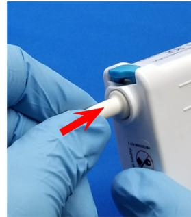
2. Push Power Cord connector in to the Battery Connector fully until an audible click is heard.
