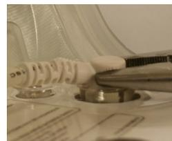
1. Firmly grasp the flat sides of the older Power Cord-to-Helmet Connector.
