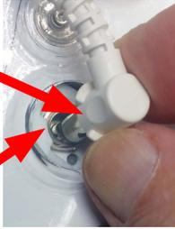
1. Align Cord notch with Helmet connector tab.
