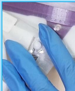
2. Snap one Lens Side Attachment Hole over FCC Side Attachment Post. Repeat for other side.
