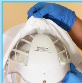
1. Snap Lens Front Alignment Hole over Helmet Front Mounting Post. Attach each Lens Side Alignment Holes over Helmet Side Mounting Posts.
